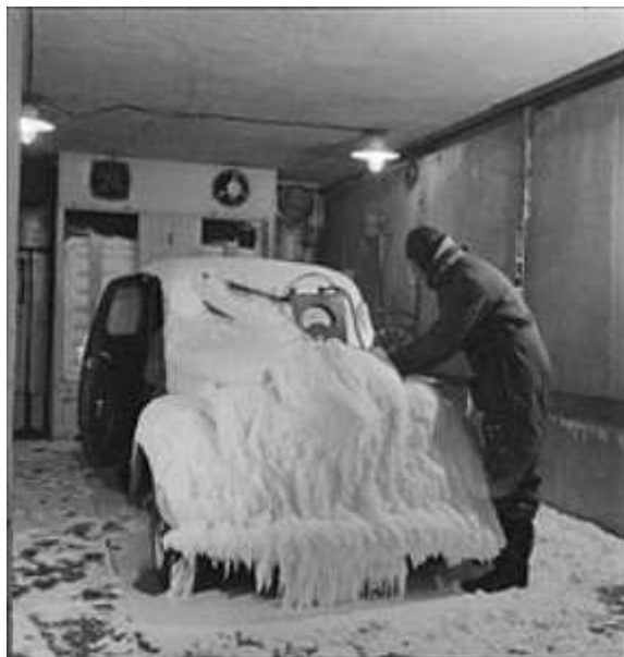
Testing the cold start capability of an engine after three days in a cold chamber. (car maker facilities in the UK, 1945)
